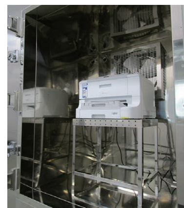
Measurement of substances released by products
