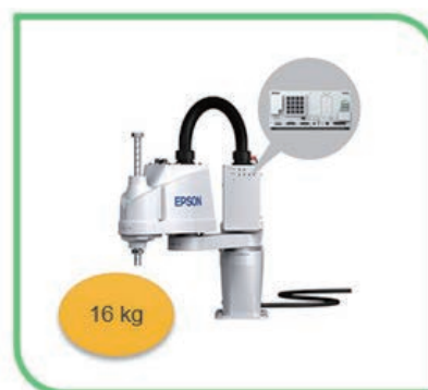
The T3 has a built-in controller
