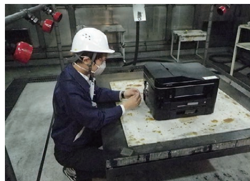
Burning test at combustion laboratory
