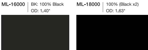
Reactive ink, Cotton 100%, Epson Edge Print PRO X2, 600x600 dpi / 2 pass Pre-treatment: PREGEN R800B, Post-treatment: steam/washing
