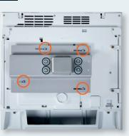
The clamp below (attached with blue-circled screws) should be shifted all the way to the RIGHT position.
