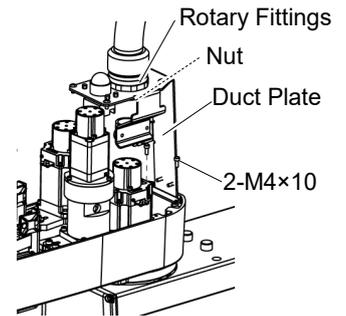
(17) Remove the rotary fitting from the metal duct.
