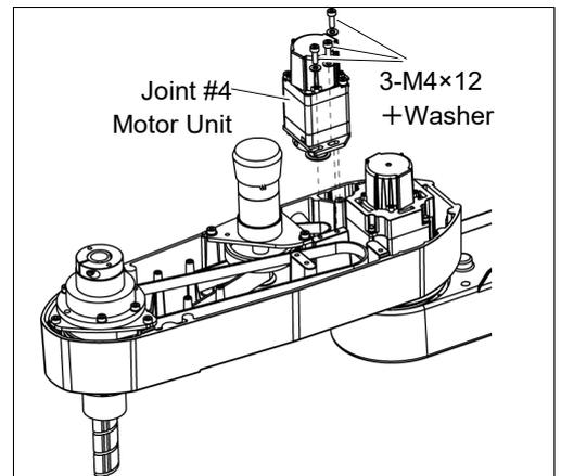
Make sure the motor unit can be moved by hand, and it will not tilt when pulled. If the unit is secured too loose or too tight, the belt will not have the proper tension.
