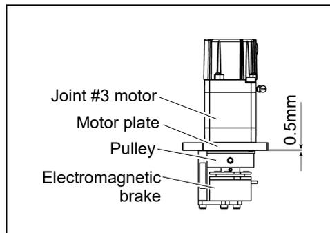
Tighten one of the set screws vertically on the flat face of the motor shaft.
