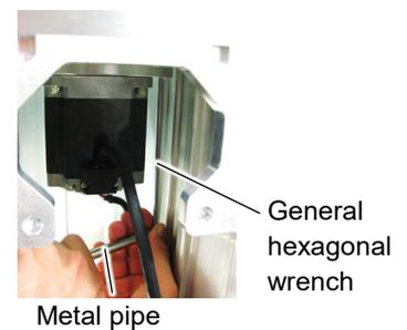
After loosening the screws, rotate the motor to pull out. If the motor is hard to pull out, pull the motor while rotating the Arm #1 slowly.
