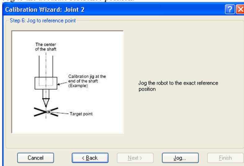
iii. Jog to the accurate reference position and adjust the position. Click the <OK> button.
