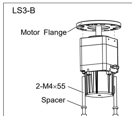
(2) Mount the waveform generator on the Joint #2 motor.
