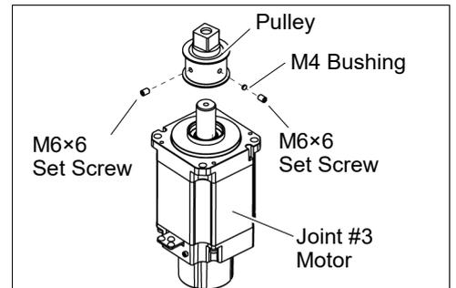
Tighten one of the set screws vertically on the flat face of the motor shaft.
