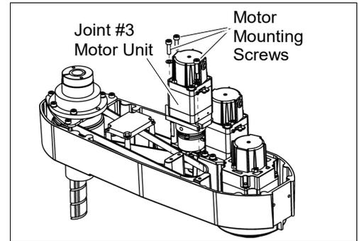
Apply the proper tension to the Z belt, and then secure the Joint #3 motor unit.
