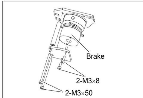
(2) Mount the brake hub to the pulley of the Joint #3 motor.
