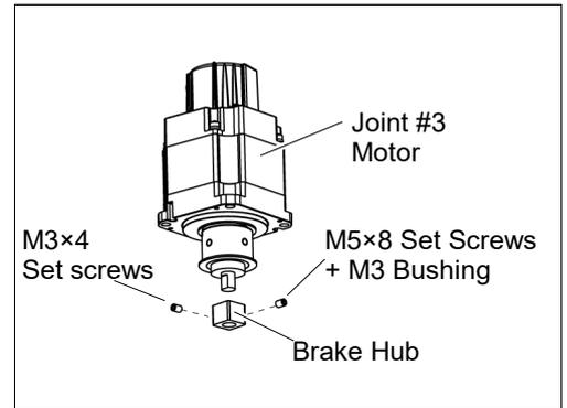
(3) Mount the Joint #3 motor to the motor plate while aligning the hub to the brake disc.
