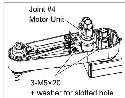
If the unit is tilted, the belt will not have the proper tension.
