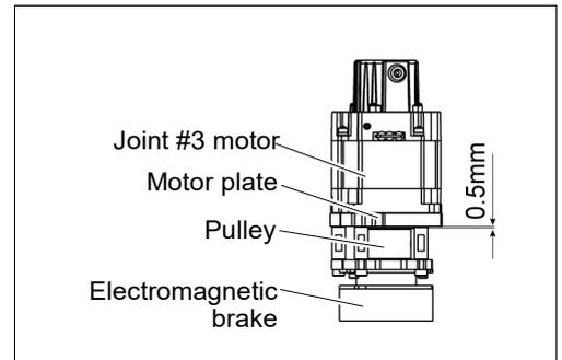
When the brake disc is not aligned, manually adjust the position by following the steps below.
