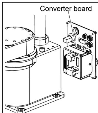
(4) Remove the converter board from the mount base.
