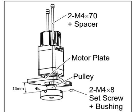
Install so that the gap between the motor plate and the pulley is 13 mm.
