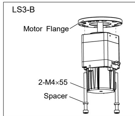
Joint #2 Motor Installation
