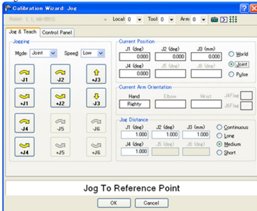
\* Position Joint #2 only and move Joint #3 to around 0 pulse.
