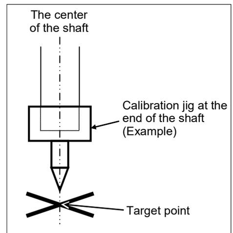
After removing the end effector and executing the calibration, install the end effector and move the Manipulator to the teaching point to verify whether there is a positional gap. If there is a positional gap, fine-tune the installation position of the end effector and teach the point again.
