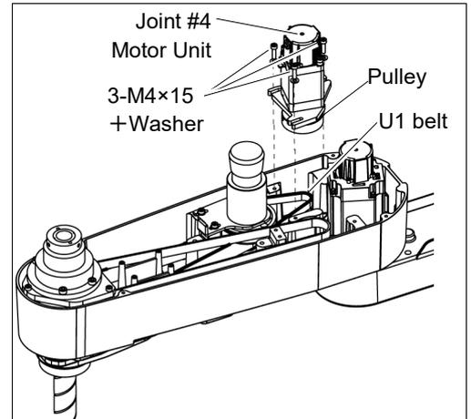
Make sure the motor unit can be moved by hand, and it will not tilt when pulled. If the unit is secured too loose or too tight, the belt will not have the proper tension.
