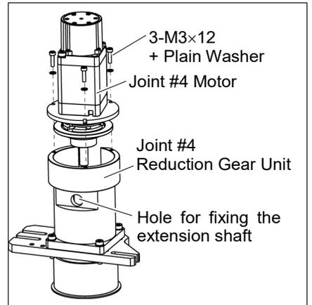
If the screw position does not match, turn the motor slightly and move until the screw fixing the extension shaft can be seen.
