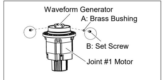
Mount the waveform generator on the Joint #1 motor.
