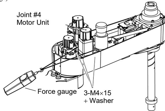
NOTE To check belt tension with the tension meter, refer to 8.4 *Checking the Timing Belt Tension (U1, U2 Belt)*.
