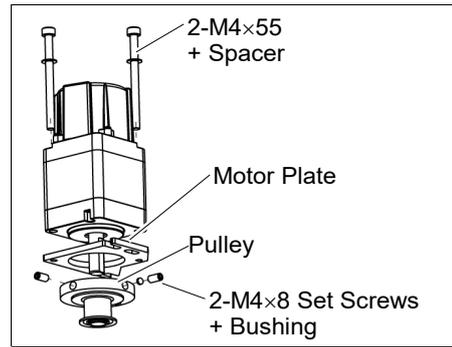
Be sure to fit the end face of the pulley to the end face of the motor shaft.
