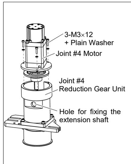
Before fixing it to the reduction gear unit, make sure to rotate Joint #4 reduction unit two or three times from the output side.
