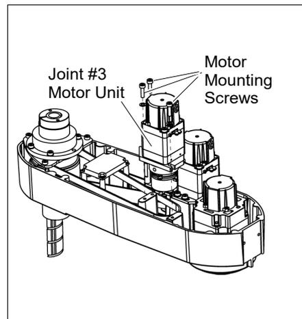
At this point, make sure that the Joint #3 motor unit can be moved by hand, and it will not tilt when pushed by tensioner. If the unit is secured too loose or too tight, the belt will not have the proper tension.
