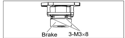
(2) Mount the brake hub to the pulley of the Joint #3 motor.
