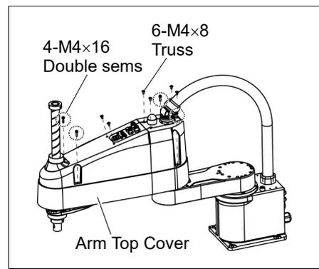
**Arm Top Cover Installation** Put the arm top cover to the arm and secure with the Arm Top Cover mounting bolts. After securing the Arm Top Cover, make sure that the lower limit mechanical stop is not touching the cylindrical part of the Arm Top Cover.
