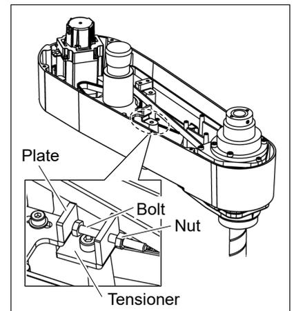
(3)-1 Loosen the nut and turn the bolt. Push in the Joint #3 motor unit.
