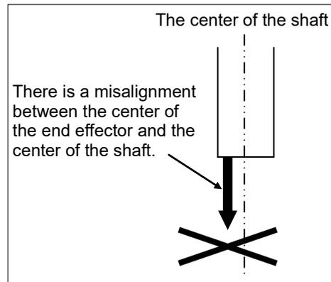
Make a calibration jig as shown in the right figure and attach it on the end of the shaft to make the center of the shaft clear.
