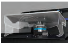
Adjust the platen height using the height adjustment.
