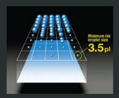
The PrecisionCore technology, as well as Variable Size Dot Technology, allow the ink droplets to be controlled to the finesse of 3.5 picolitres, ensuring precision in every print.
