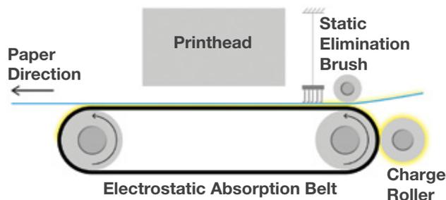
The WorkForce Enterprise uses an electrostatic transport belt that ensures the paper is completely flat, enabling the smoothest of gradients and consistently sharp images.
