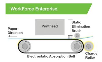
The WorkForce Enterprise uses an electrostatic transport belt that ensures the paper is completely flat, enabling the smoothest of gradients and consistently sharp images.
