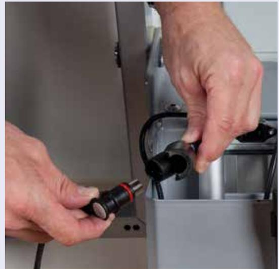
Plug in the remote control into the remaining connector.
