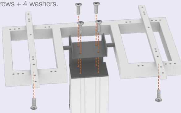
Make sure to run the two cables exiting the column through the cut out of the board frame before securing the 4 bolts.
