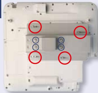
Carefully place the projector plate on top of the spacers and washers and secure the plate with 4 x allen head screws M4 x 20 (0.15" x 1 3/4").
