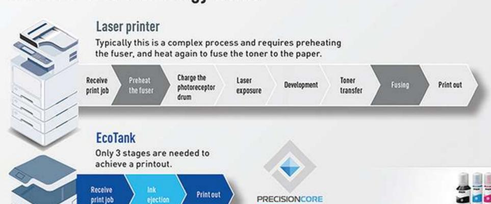
Epson Heat-Free Technology does not require heat in the ink ejection process. Instead pressure is applied to the Piezo element, which flexes backwards and forwards firing the ink from the printhead. This means printer parts last longer and energy consumption is reduced, saving energy, time and money in the process.
