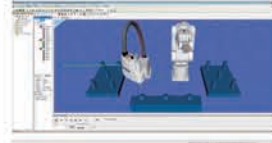
3D simulator for work cell layout and toolpath program testing
